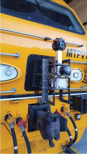
Appendix 2 – LIDAR fitted in Mechanised Track Patrol Vehicle
