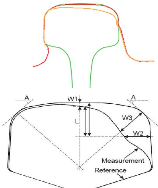
Figure 4 - Rail Profile Recording against Template (above)
