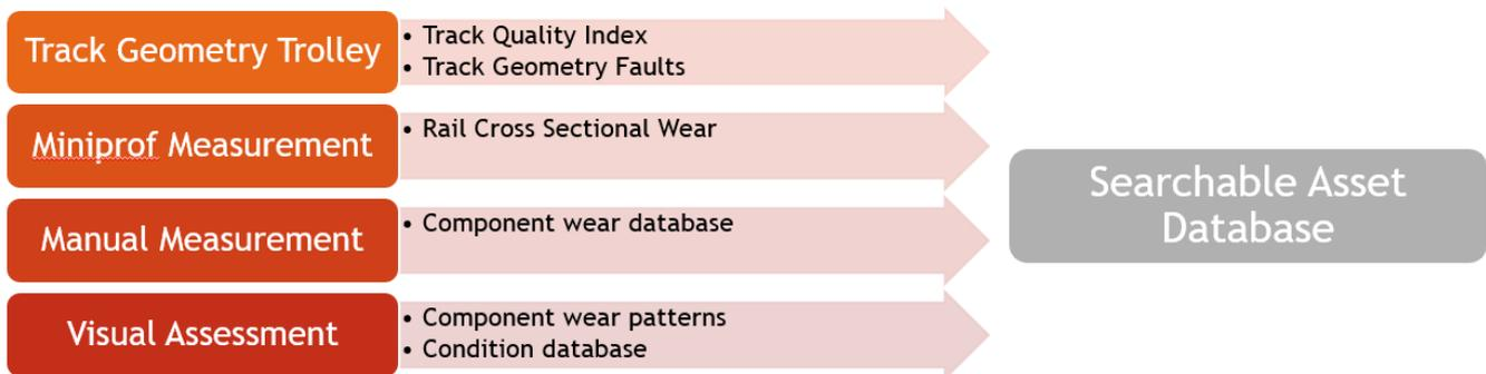
The data from the track geometry trolley was parsed for track faults, and a Track Quality Index was produced. This was then compared and scored against a control turnout TQI and a track geometry score was assigned to each turnout.
