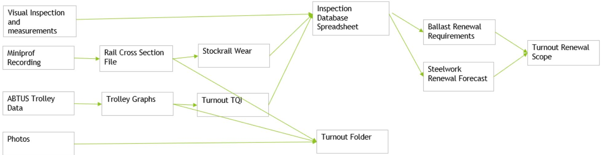
Figure 5 - Turnout Assessment Model Data Flow
