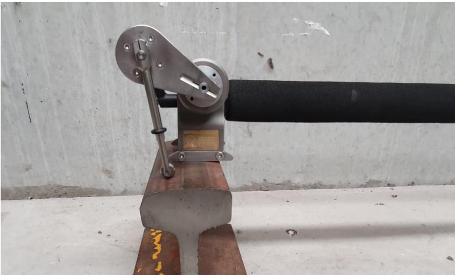
*Figure 1 - Miniprof rail profile instrument*
