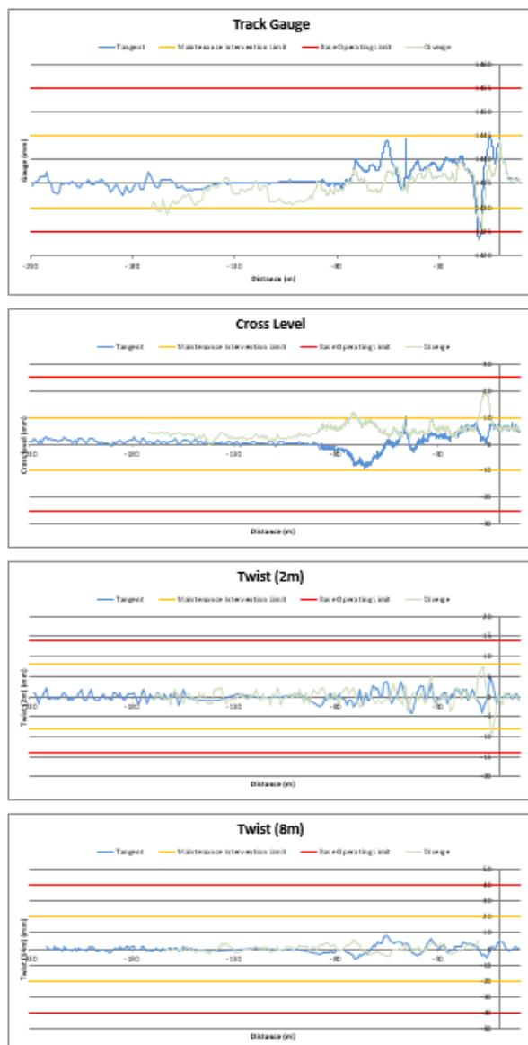
Figure 3 - Track Geometry Data - Graphed for Tangent and Diverge
