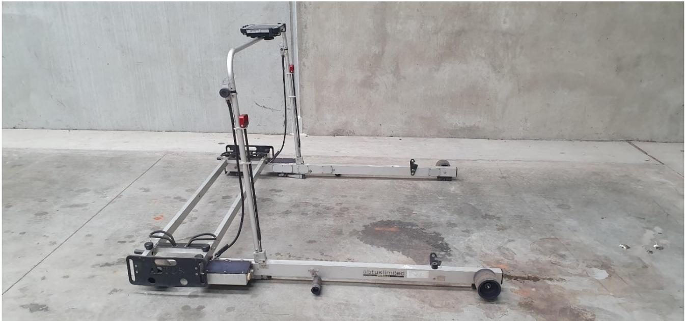
Figure 2 - ABTUS 4530 Track Geometry Trolley
