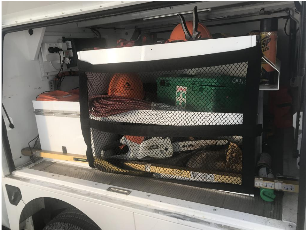
City South Incident Response ute with inverter and battery charger on the left
